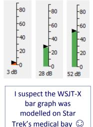
The bar graph bar should normally be green, showing acceptable levels. If it is red, the level is probably too high (causing distortion, apparently wide signals and poor copy) or too low (no input meaning no signals to copy!).
